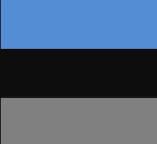
Deckschicht<br>3.5 cm<br>Binderschicht<br>7 cm<br>Tragschicht<br>8 cm | OK Fahrbahn<br>↓<br>
